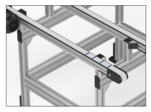
Heavy objects with small contact surface may create high loads on a very short portion of the belt. The smallest unit defined is the load per belt tooth. Exceeding this load concentration level may lead to excessive wear of both the belt and the guiding profile. See <u>Table 1</u>.
