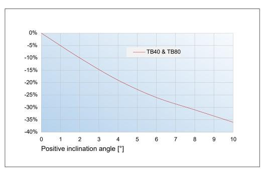
TB40 & TB80 load reduction at inclination [%]
