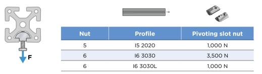
Note: The above stress limits have been determined on samples subjected to pull-out tests.
