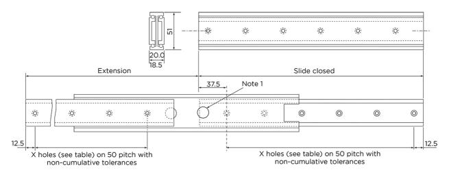
Note 1: 15 mm dia. holes in centre beam allow easy access to fixing holes. M5 countersunk head screws to BS4183 are recommended for fixing.
