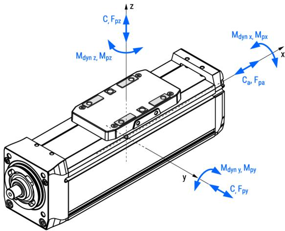
The moved mass is already considered in the equation for calculating the mass of the linear unit  $m_{\text{MGBS}}$  and the mass moment of inertia  $J_{\text{MGBS}}$ . The moved mass includes the mass of the carriage together with the ball nut.
