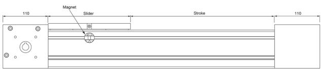
Total length = Stroke + slider + 220 Stroke: We recommend to add min. 50 mm to the nominal stroke (stroke = nominal stroke + 50 mm)
