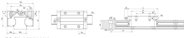
\*\*E: Size 15 delivered with straight standard nipple. Size 20 – 55 delivered with angled standard nipple.
